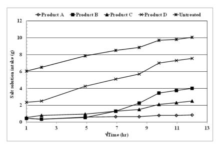
**USP-200** is product 'A' in the above test result for Chloride solution ponding over 90 days. It shows negligible Chloride intake compared with treatment products B, C and D by other manufacturers.
