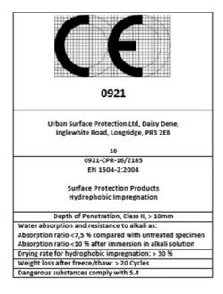
**USP-200** has been tested compliant to EN1504-2. Chloride Resistance (EN1504-7) has been determined by the salt ponding method.
